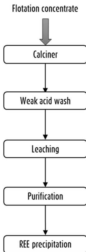
Figure 1 – Simplified Montviel Hydrometallurgical process to extract REE
