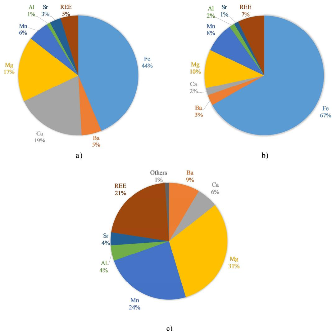
Figure 2 – Effect of pre-treatments on HCl consumption of REE extraction, a) Total HCl Consumption during direct leaching of Montviel FC = 293 kg HCl (100%)/t ore b) HCl Consumption after weak acid wash = 191 kg HCl (100%)/t ore, c) Total HCl Consumption affected by two treatments (weak acid wash and optimised REE leaching), 63.2 kg HCl (100%)/t ore
