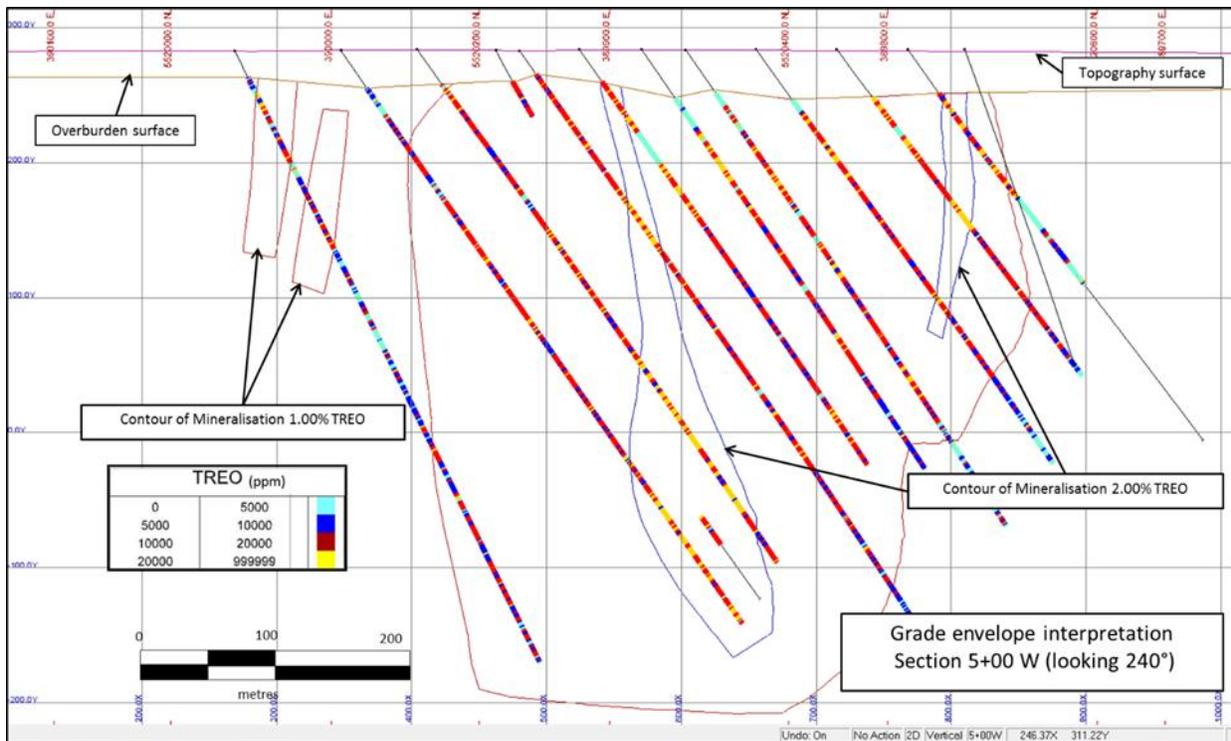
**Figure 14.5: Resulting Mineralised Solids, Montviel Project**
