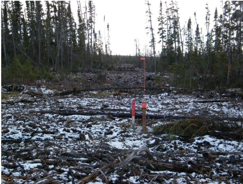
**Figure 12.6: Drill Casing Identifying Drill Hole Location**
